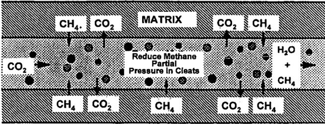
Figure 2 CO<sub>2</sub>-enhanced coalbed methane recovery mechanism.
