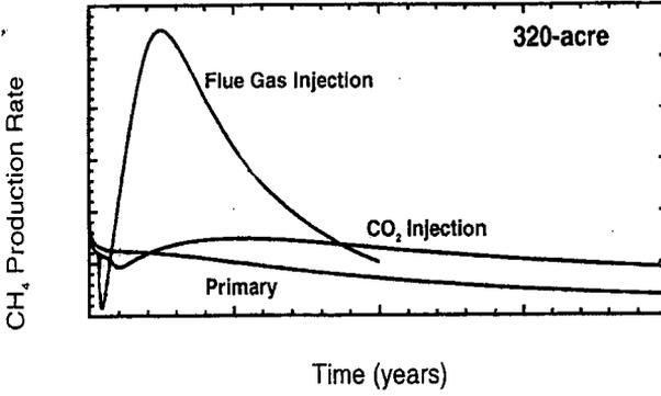
Figure 3 Coalbed methane production rate over time for primary recovery and as a result of pure CO<sub>2</sub> and flue gas injection.
