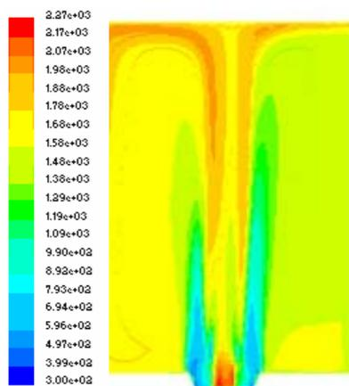
**Figure 2.** Low-NO<sub>x</sub> case temperature profile (axial surface)
